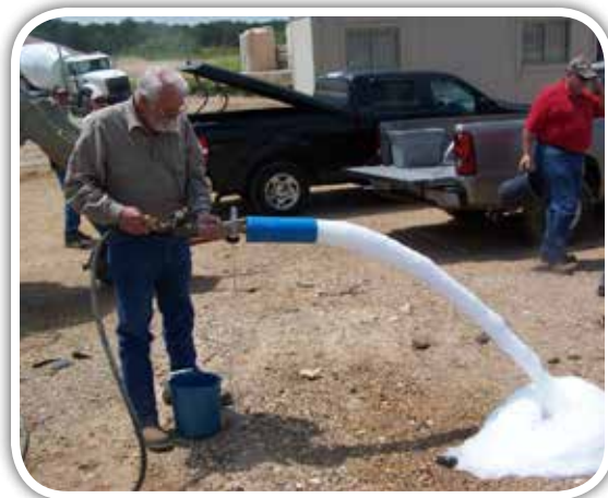
To produce cellular grout, a concentrated foaming agent is required in combination with various types of foam generating equipment. This equipment may generate foam via air pressure or water pressure.
