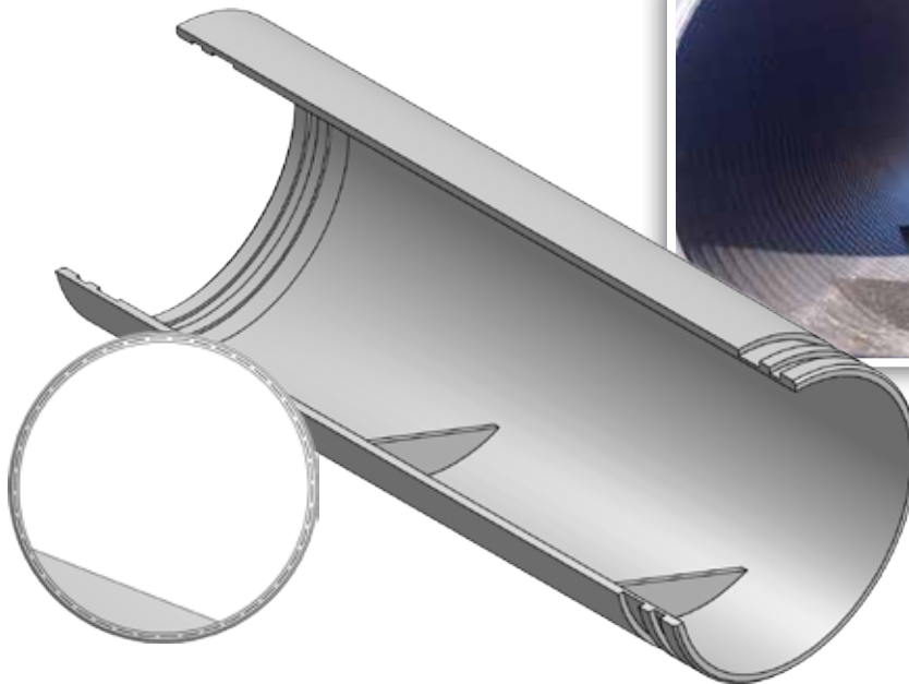
Baffles are placed off center from the invert or flowline of the culvert and remain on one side of the culvert and do not alternate.
